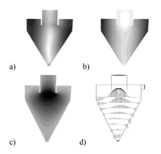
Figure 3. Contours of a) velocity b)static pressure, c)turbulent kinetic energy, d)velocity vertical vectors.
